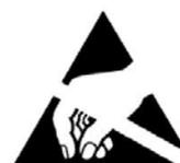
The product is containing electronics which may be sensitive to electrostatic discharges (ESD) as well as mechanical stress. To avoid damages, any open circuit board like LED-modules should never be directly touched by hand or by a tool. This is valid both during installation and normal maintenance.
