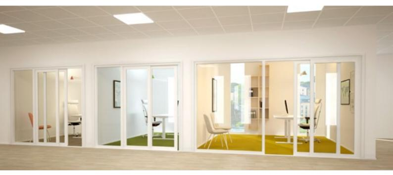
e-Sense Tune allows environments with different colour temperatures to be created. First office 4000 K, second office 6500 K and third office 3000 K.
