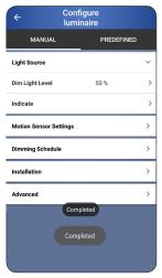
Completed is displayed when the luminaire has flashed.
