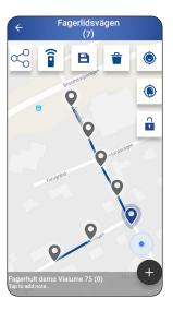
A link is missing here between the luminaires; this configuration will not work.
