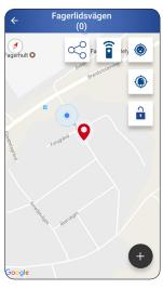
Luminaire that is difficult to communicate with is displayed with a red position pin.
